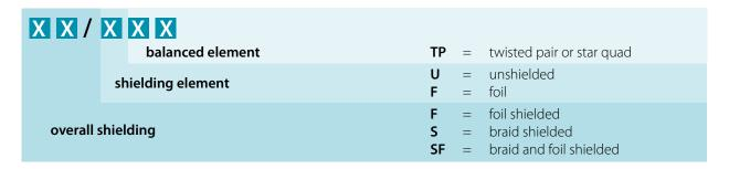
**Examples** SF/UTP = overall braid and foil shielded cable / with unshielded balanced elements
